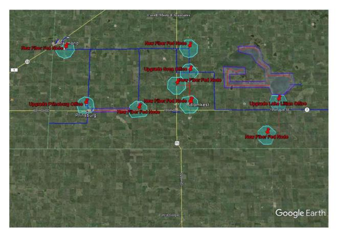
Blue shaded areas denote 25/3 serving areas established by placing fiber to new nodes and shortening existing customer loops. Purple shaded area denotes 25/3 serving area by placing fiber to the home. Blue lines denote existing Frontier fiber and red lines denote new fiber that will be placed
