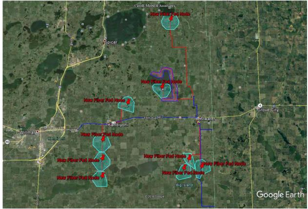
Blue shaded areas denote 25/3 serving areas established by placing fiber to new nodes and shortening existing customer loops. Purple shaded area denotes 25/3 serving area by placing fiber to the home. Blue lines denote existing Frontier fiber and red lines denote new fiber that will be placed.
